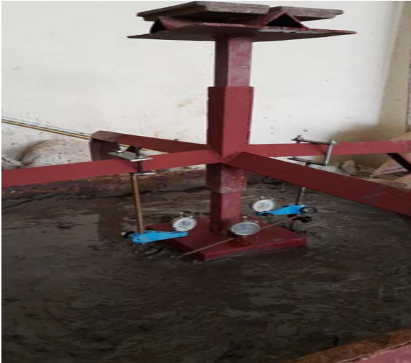
Photo (2): Test Footing and Loading System.
