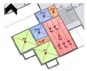
Fig. 5. Network module for 12 measuring points of the apartment
