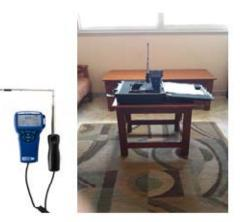
Fig. 6. Air velocity meter 9545-A and the field of study
