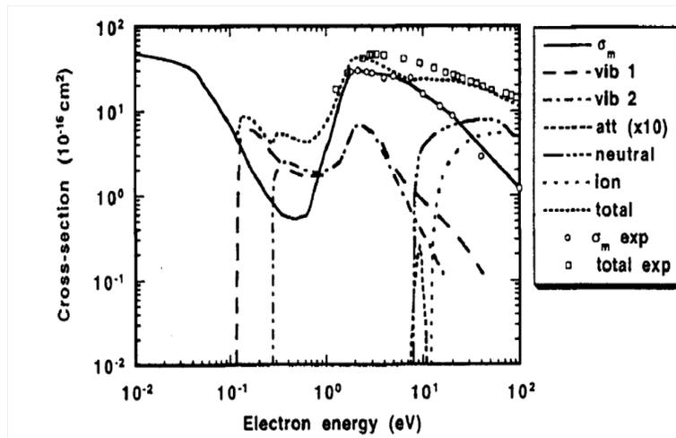
Fig. (3) Set of cross sections of electron impact on SiH<sub>4</sub> : The experimental data of **Tanaka** et al. for the elastic (momentum-transfer) cross-section and of Mori et al. for the total cross-section are shown for comparison
