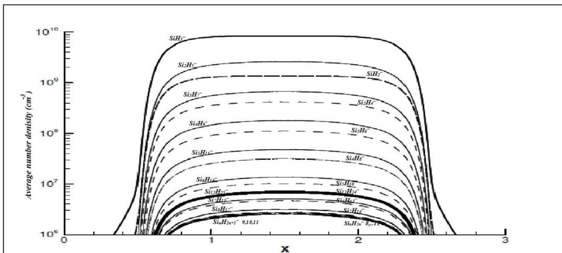
Fig. (9) Anion silyle ( $\text{Si}_n\text{H}_{2n+1}^-$  in solid lines) and silylene ( $\text{Si}_n\text{H}_{2n}^-$  in dashed lines) density profile.
