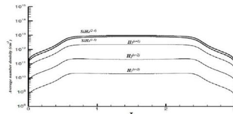
Fig. (8) Density profile of Hydrogen and Silane excited states
