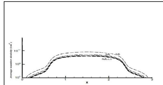
Fig. (6) Density profile of neutral radicals silylene Si<sub>n</sub>H<sub>2n</sub> in Silane discharge.
