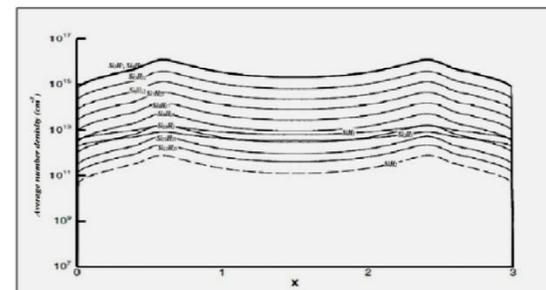
Fig. (7) Density profile of neutral radicals silyl (Si<sub>n</sub>H<sub>2n+1</sub>) in Silane discharge.
