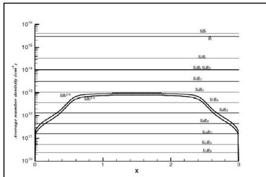
Fig. (5) Density profile of neutral background molecules, Si<sub>n</sub>H<sub>2n+2</sub> and excited molecules of SiH<sub>4</sub>.
