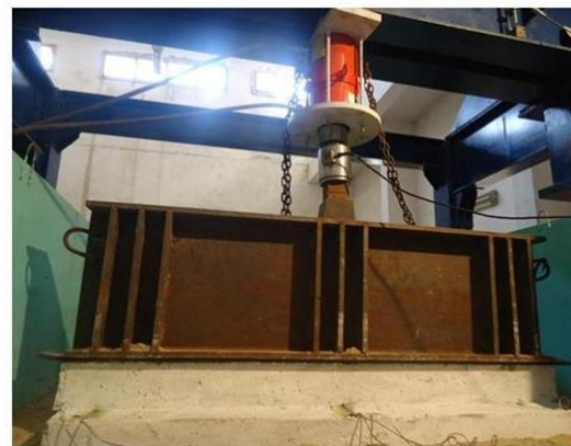
Photo (2): Sample Loading and Strain Gauges Arrangement.
