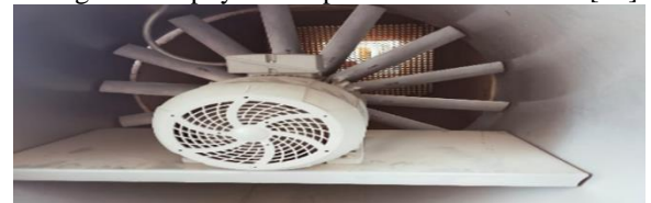
Fig.38. The motor used to produce the air flow using an axial fan
