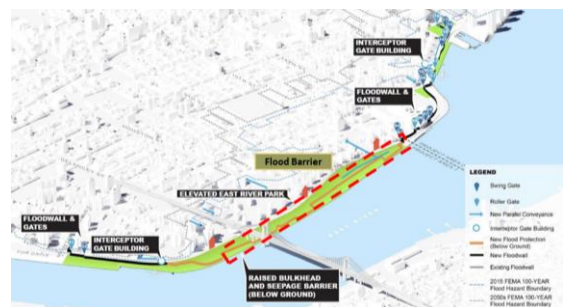
Figure 5 The East Side Coastal Resiliency project protects 110,000 residents of Manhattan's Lower East Side from potential coastal and tidal floods by constructing a continuous 2.4-mile barrier with berms, flood walls, flood gates, and raised parklands [40].
