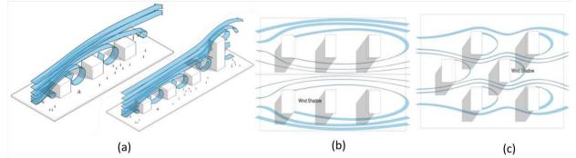
Fig. 18. The effect of buildings hight on wind shadow pattern (a) – wind shadow of parallel urban pattern (b) – wind shadow of reciprocal urban pattern (c) [Author]
