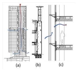
Fig. 15. Air movement through: atrium (a) – solar chimney (b) – double skin façade (c) [51, 52]
