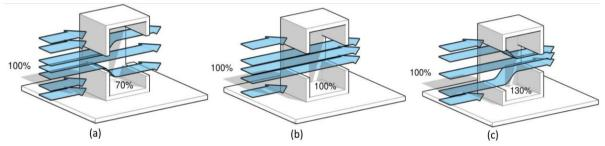
Fig. 22. Variation in air flow rates within a space due to variation in the air inlet and outlet size -(a) the inlet is smaller than the outlet -(b) the inlet and outlet are the same -(c) the inlet is bigger than the outlet size [Author]
