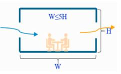
Fig. 11. Depth of the space compared to its height in cross-ventilation strategy [33]
