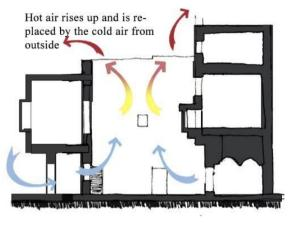
Fig. 16. Air movement inside the courtyard [35]
