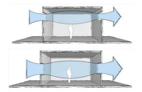
Fig. 21. High-level openings result in bad ventilation (top) - Two opposite openings at a human level for good ventilation (bottom) [Author]
