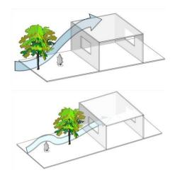
Fig. 17. Using trees to direct air away (top) and into (bottom) the building [Author]
