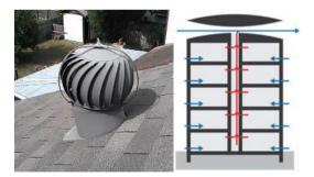
Fig. 13. Air movement through: Rotating Ventilator (left) - Venturi roof (right) [37, 49]
