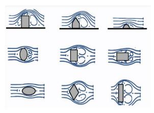
Fig. 19. Effect of building shape on wind pattern [54]
