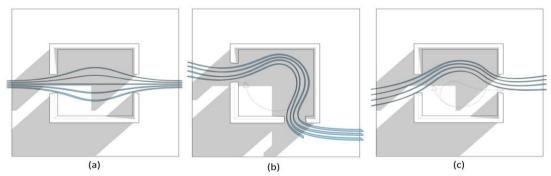
Fig. 20. Two opposite openings and vertical wind (a) - Two adjacent openings and vertical wind (b) - Two opposite openings and tilted wind (c) [Author]
