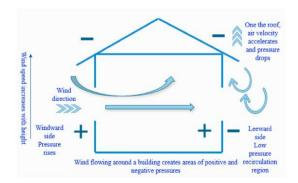
Fig. 6. Airflow caused by wind-driven force [33]
