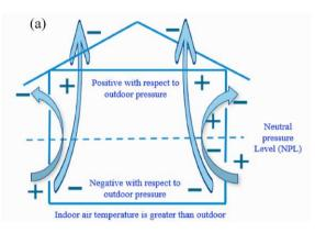
Fig. 7. Airflow caused by the stack effect [33]
