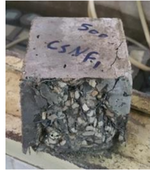
Photo (1): Failure mode for a concrete specimen of 2 % steel fibers with nano and micro silica under the compression test
