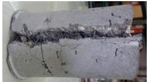
Photo (2): mode of failure for a concrete specimen of 2 % steel fibers with nano and micro silica under the splitting tensile strength test.
