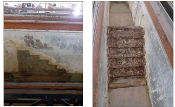
(3.a) (3.b) Figure 3 The experimental gabion stepped spillway model
