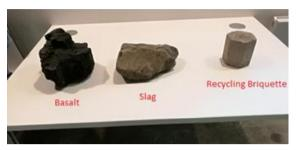
Figure 3: The essential components of rock wool tiles (Source: Technical training for the researcher 2018)
