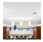
Figure 2: Photo of a mineral fiber suspended ceiling (Source: Armstrong Catalogue page 226)
