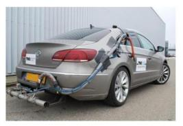
Fig. 4. Portable emissions measurement system [72].
