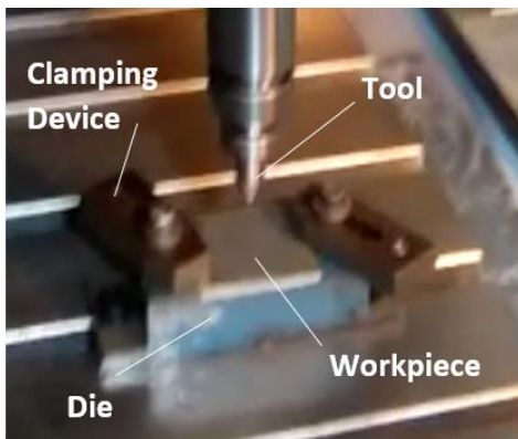
Figure 3. The experimental setup for TFD carried out in the present investigation.
