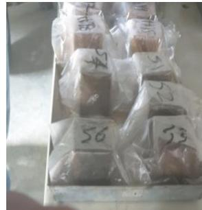
c) Covered specimens inside moulds
