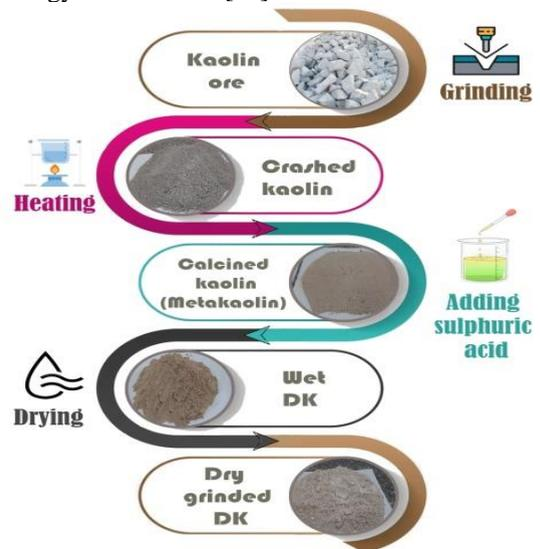
Fig.1: Production of alum and de-aluminated metakaolin [8]
