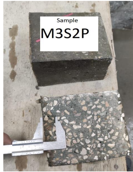
Fig.17 Split M3S2P specimen at room temperature.
