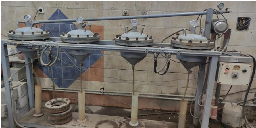
Fig. 4 Water penetration test of concrete
