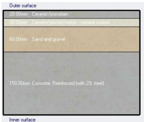
Fig. 7. Construction Material presentation in DesignBuilder
