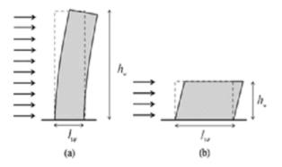
Figure 2 – a) Flexural deformation, b) Shear deformation Paulay et al. (1995).
