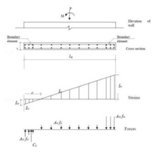
Figure 1 – Wall section equilibrium under flexural and axial loads Paulay et al. (1995).
