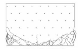
Figure 4 – Flexural failure of RC walls Greifenhagen et al. (2005)
