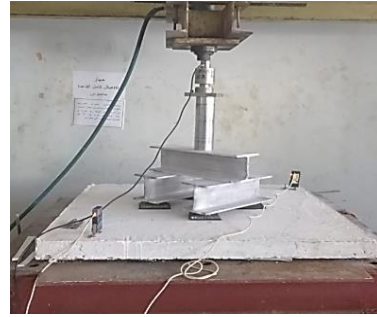
Fig.5. Loading arrangement and test setup
