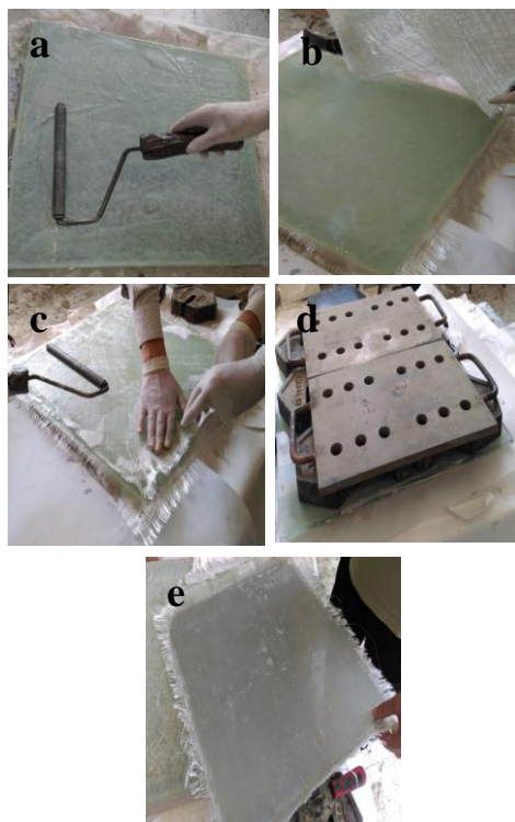
Fig. 2. Steps for specimens manufacturing
