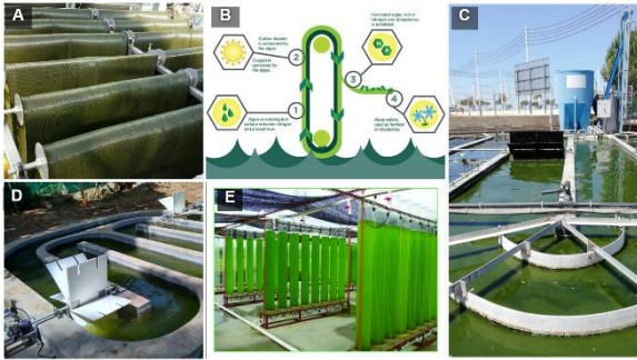
Figure 4: Microalgae Cultivation Systems for Wastewater treatment, Columbus. A, B) Revolving Algal Biofilm (RAB) Wastewater Treatment C) High-Rate Algae Ponds in Aqualia, Spain., D) Race way algal pond, and E) closed photobioreactors, Foshan city, South China.
