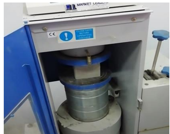
Fig. 3. Sample of Cubes Under Compressive Force.
