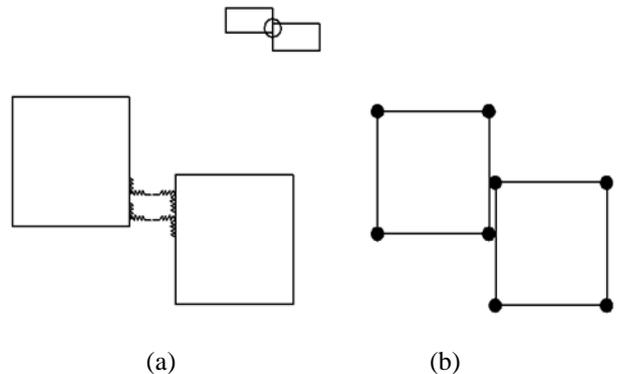
Fig. 4. Element Connectivity; (a) AEM (connectivity via springs), (b) FEM (no connectivity) [12]
