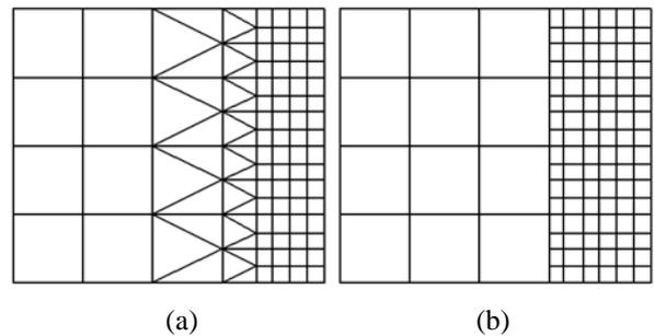
Fig. 3. Transition from Large Elements to Small Elements in: (a) FEM, (b) AEM[12]
