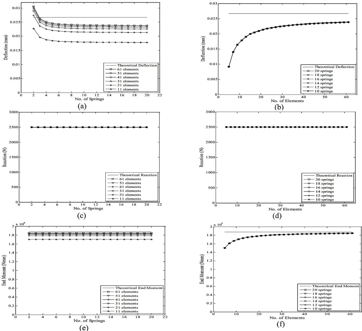
Fig.12. Results (a) deflection vs number of springs, (b) deflection vs number of elements, (c) reactions vs number of springs, (d) reactions vs number of elements, (e) end moment vs number of springs, (f) end moment vs number of elements [13].
