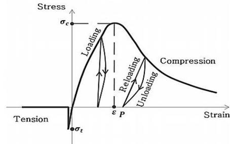
Fig. 6. Axial stress-strain curves for concrete [14]
