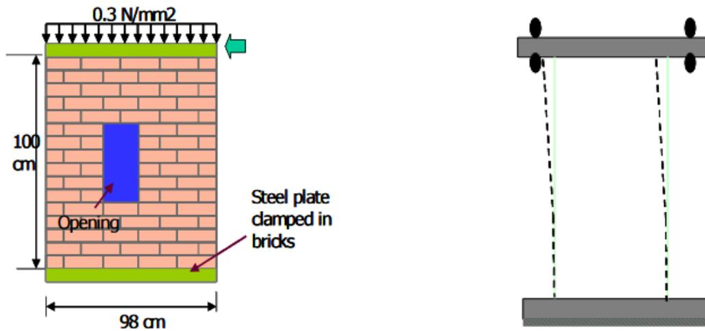
Fig. 15. Test wall and schematic boundary condition[19].
