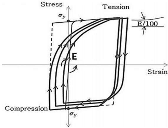
Fig. 7. Axial stress-strain curves for steel [14].
