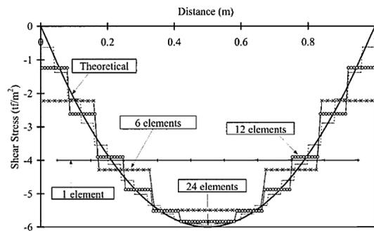
Fig.10. Shear stress distribution at column base [1, 2]
