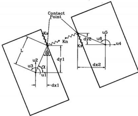
Fig. 1. Element shape, contact point and degrees of freedom for two elements [5]
