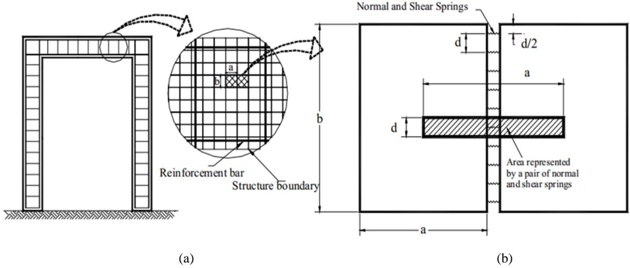
Fig. 5. Modelling of structure in AEM: (a) Element generation for AEM, (b) Spring distributions and area of influence of each spring [10]
