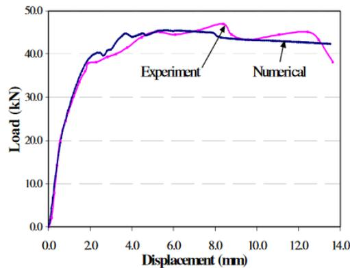
Fig. 17. Comparison of experimental and numerical analysis results[19].
