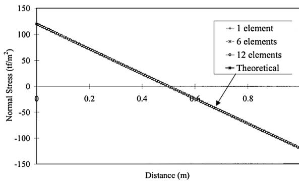
Fig.9. Normal stress distribution at column base [1, 2].
