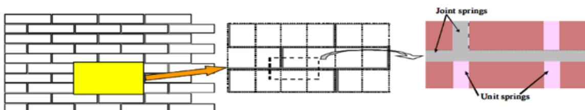
Fig. 14. Masonry discretization[18].
