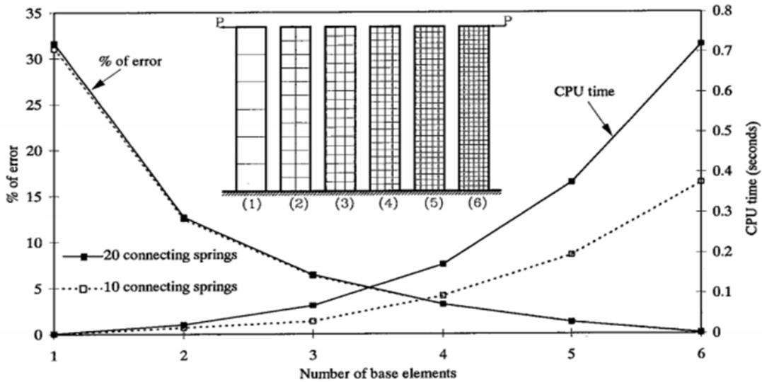
Fig. 8. Relations between number of base elements, ratio of error and CPU time [2, 3]
