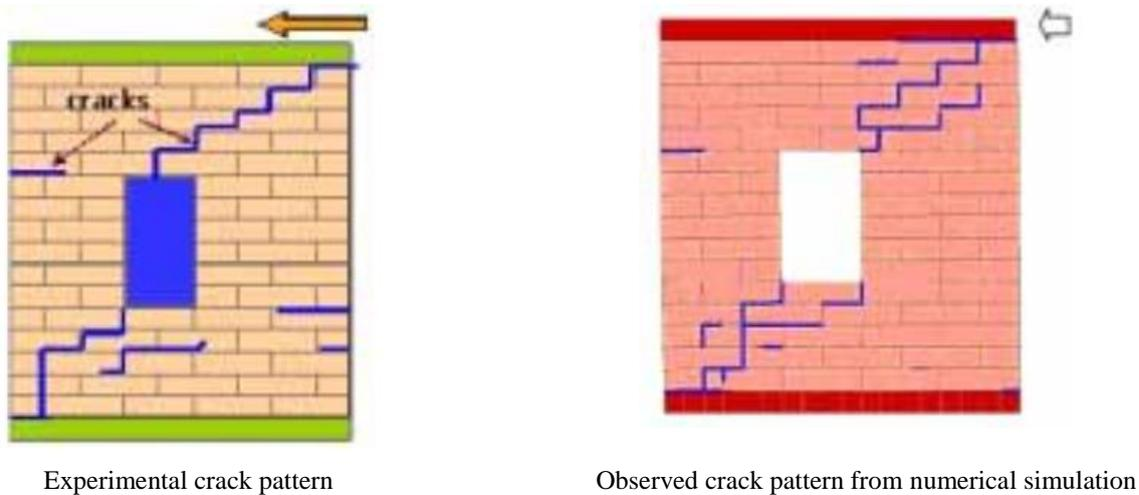
Fig. 16. Crack pattern observed in test and obtained through analysis[19].
