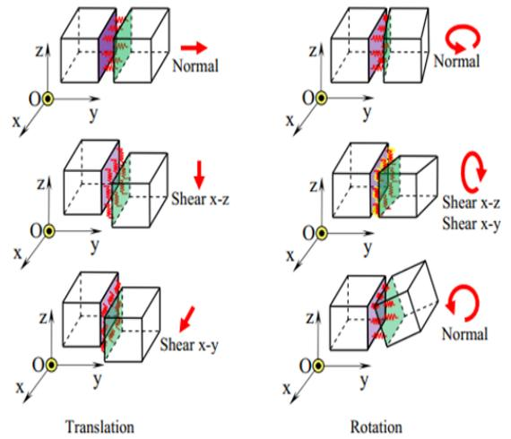
Fig. 2. Six degrees of freedom in 3-D analysis and connecting springs [11]
