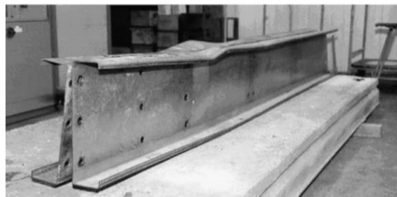
Fig.7. Experimental Channel Buckling Failure
