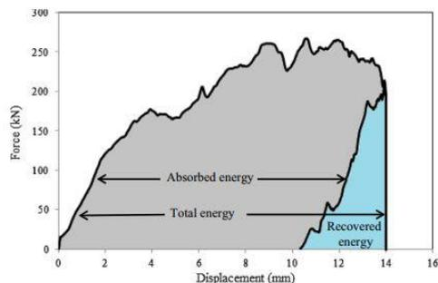
Fig. 3. The impact force – displacement curve. ( Remennikov et al, [3])
