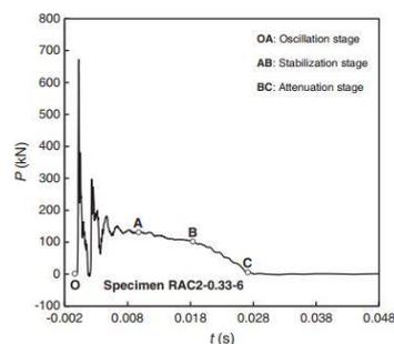
Fig. 2. Typical time history of impact loads.(Yang et al, [12])
