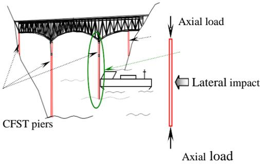
Fig. 1. A graphical view of the collision between the ship and the bridge. (Wang et al, [7])
