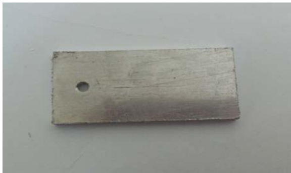
Fig.2: Aluminum alloy with purity 99.5%
